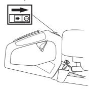
Start the engine and make sure the engine stops when you move the stop switch to the stop setting.
